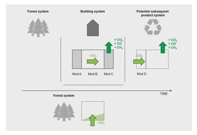
Figure 4.12: The time dependent approach, considering that trees regrow after harvesting. The dotted lines indicate the product systems which fall outside the building system boundaries. Source: Hoxha et al (2020b).
