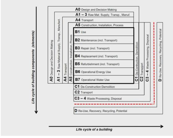
Figure 4.5: Alternative model of the life cycle of buildings and building components (Lützkendorf 2019)
