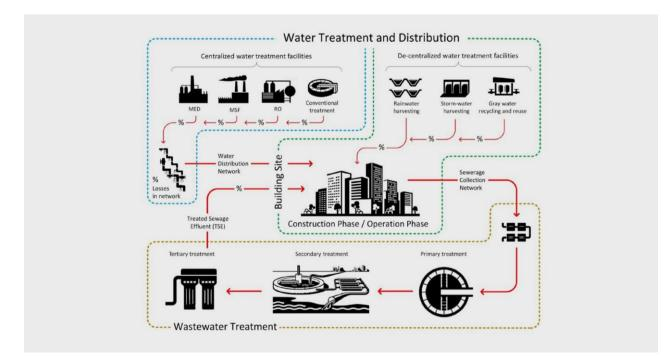
Figure 4.29: Main stages of the built environment hydraulic cycle: water treatment and distribution, water use and wastewater treatment. (Source: Mannan and Al-Ghamdi (2020)).
