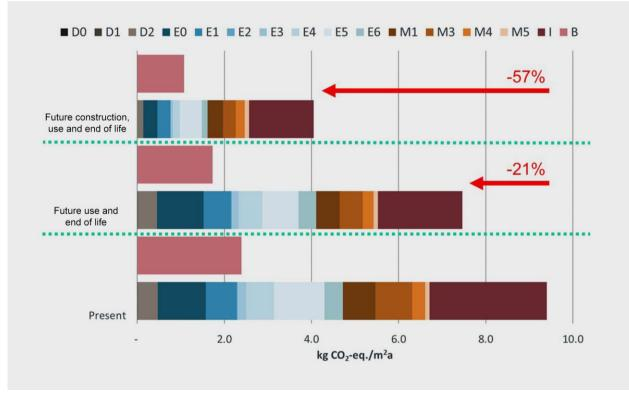
**Figure 4.7:** The greenhouse gas emissions per m2 and year of the residential building Rautistrasse of building construction and dismantling are reduced by 57%. Note. The residential building Rautistrasse has 104 apartments and has been built according to the Minergie Eco standard (for short description see: A72 report by Birgisdóttir and Stranddorf (2022), case study 05; for a detailed description see: Alig et al., 2020<sup>23</sup>).
