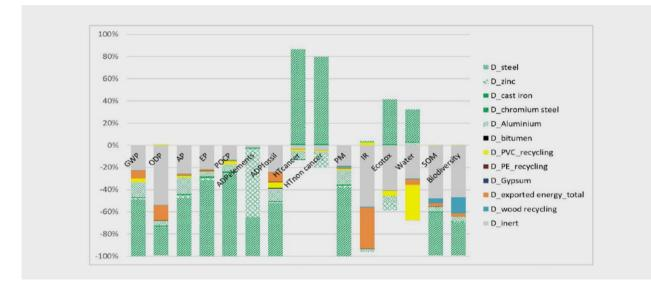
**Figure 4.31:** An overview of the contribution of each type of material to module D for the sand-lime brick framed building as an example. (Source: Delem and Wasties 2019a). Note: Even though no metal structure was considered among the building variants, and technical installations were excluded from this case study, metals and especially steel represented a major contributor to module D.
