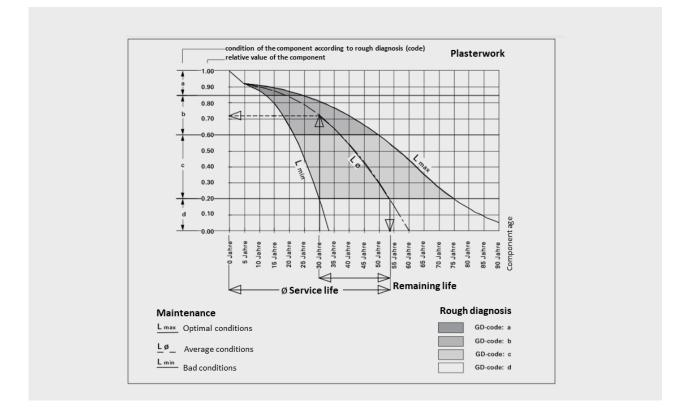
**Figure 4.38.** Example of an aging diagram of a component to identify the remaining service life value (Source: adapted from Bundesamt für Konjunkturfragen (1994)).
