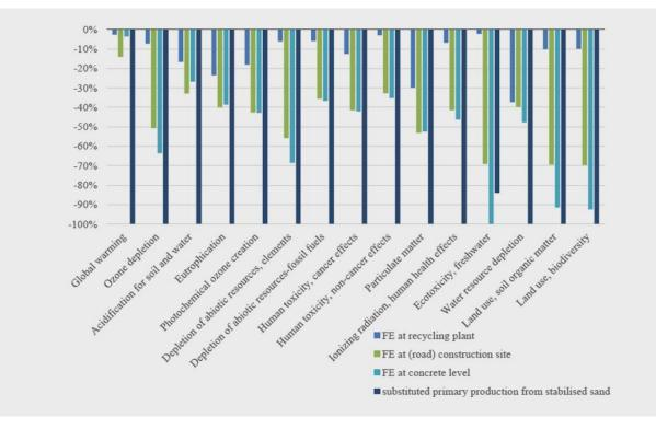
Figure 4.33: Net benefits reported in module D of concrete when recycled aggregates substitute crushed limestone and the point of functional equivalence (FE) is set at different levels, or when recycled aggregates substitute stabilised sand (Source: Delem and Wasties (2019b))
