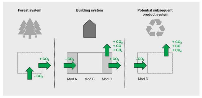
Figure 4.9: The -1/+1 approach to model biogenic carbon uptake and release. The dotted lines indicate the product systems which fall outside the building system boundaries. Source: Hoxha et al (2020b).
