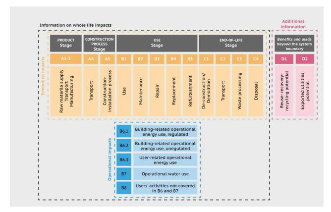
Figure 4.4: Modular approach of building life cycle impacts, distinguishing between the impacts arising from embodied (green dotted line) and operational aspects (blue dotted line). Adapted from EN 15643:2021.
