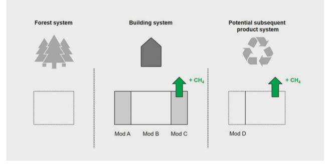
Figure 4.8: The 0/0 approach to model biogenic carbon uptake and release. The dotted lines indicate the product systems which fall outside the building system boundaries. Source: Hoxha et al (2020b).
