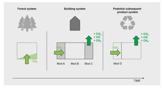
**Figure 4.11:** The time dependent approach, considering that trees grow before the use of the harvested wood product. The dotted lines indicate the product systems which fall outside the building system boundaries. Source: Hoxha et al (2020b).
