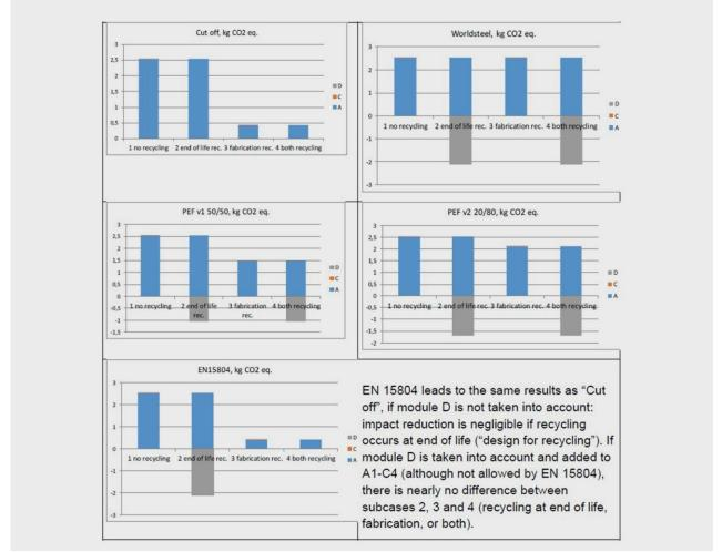
Figure 4.32: Presentation of four subcases depending on whether steel is recycled at fabrication, at EoL or not at all (Source: Annex 72 case study on modeling recycling).
