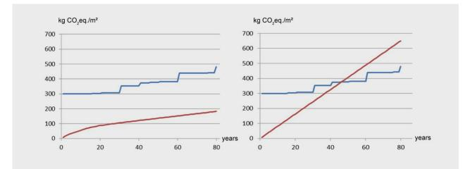
**Figure 4.6:** Embodied GHG emissions (blue line) and operational GHG emissions (red line) for an office building calculated over 80 years reference study period using forecasting scenario vs. static energy approach only for the operation part (Birgisdottir & Stenholt Madsen 2017).
