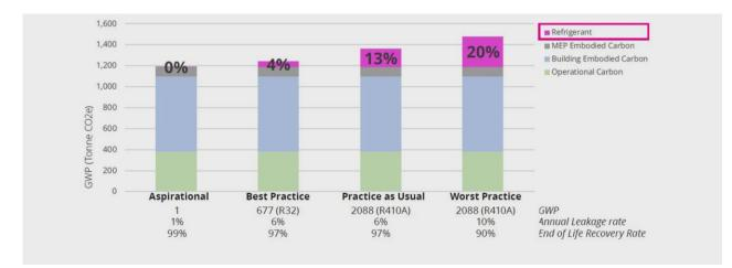
**Figure 4.14:** Whole life carbon emissions over 30 years of a US low energy office building (2,000 m<sup>2</sup>) using a VRF system. Depending on the refrigerant used, its leakage rate and recovery at end of life, refrigerant can have a different impact on global warming. (Source: Hamot et al., 2020).
