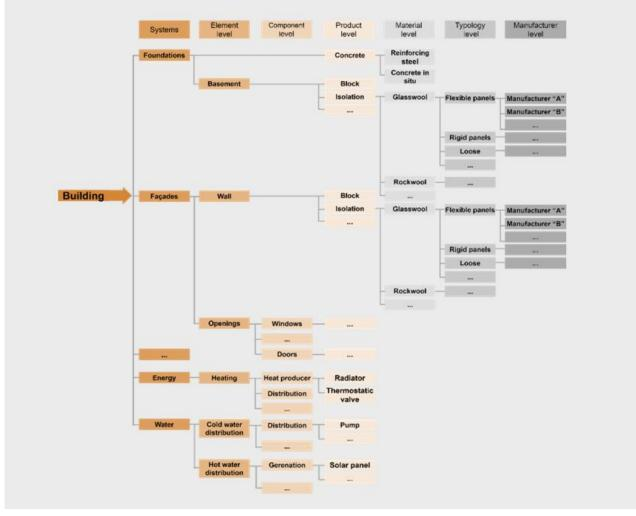
Figure 4.3: An example for a building decomposition model (source: A72 report by Passer et al. (2022))
