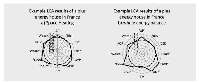
Figure 4.25: Impacts of electricity use in a Plus energy house in France (Roux et al. 2016b), Comparison between an hourly mix (plain line) and a yearly average mix method (dotted line).
