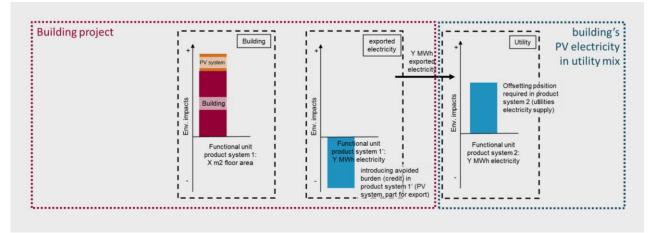
Figure 4.28: Approach 3: Allocation of 100 % of the environmental impacts of onsite energy production and 100 % of potentially avoided emissions in Module D2, outside the system boundary of the building but as part of the building project.
