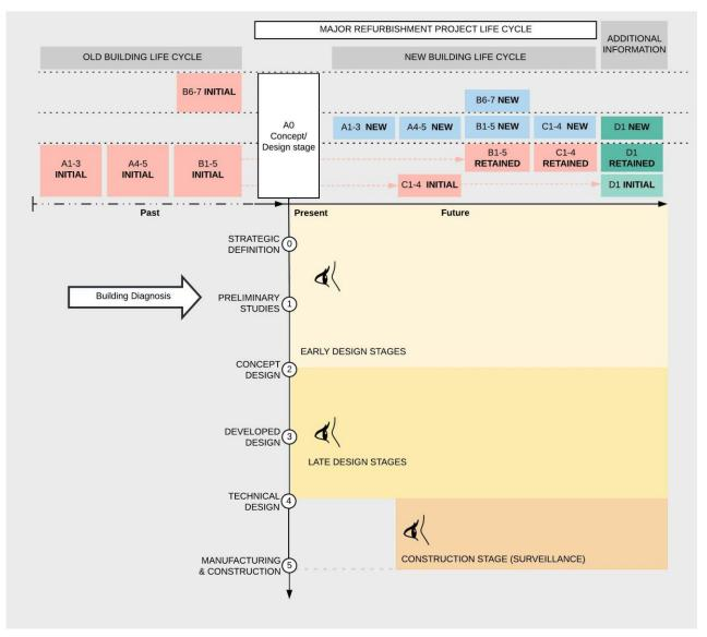
**Figure 3.3:** Relationship between the typical project and design steps for a building to be refurbished or repurposed and the building's physical life cycle (authors' own illustration). Note: The designer should consider the entire building life cycle in all steps of the design process in the A0 stage to the extent possible based on availability of appropriate data.
