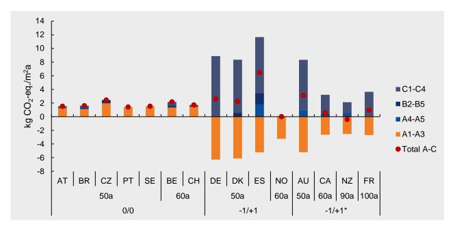
Figure 4.10: Greenhouse gas emissions of the superstructure of a Canadian wooden building assessed (see description of the case study and more results in Ouellet Plamodon et al. (2022)).
