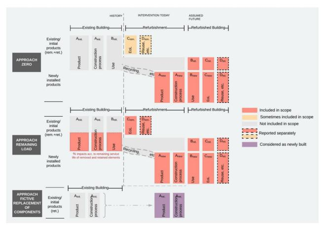
Figure 4.39. Visualisation of the three allocation approaches of the pre-refurbishment impacts associated with initial structure further used in a refurbished building (Source: Balouktsi and Lützkendorf 2022). Note: newly added is denoted as "new", removed is denoted as "rem." and retained as "ret.".
